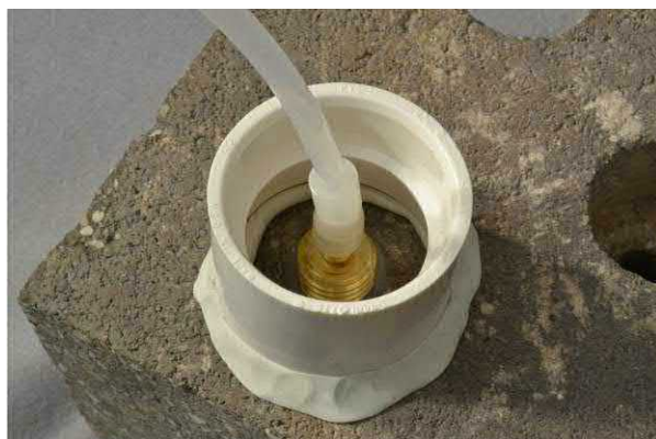
Figure 6. Water dam used for leak detection.
