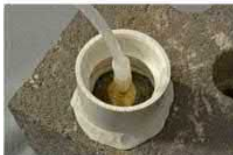
Figure 9: Water Dam Used for Leak Detection
